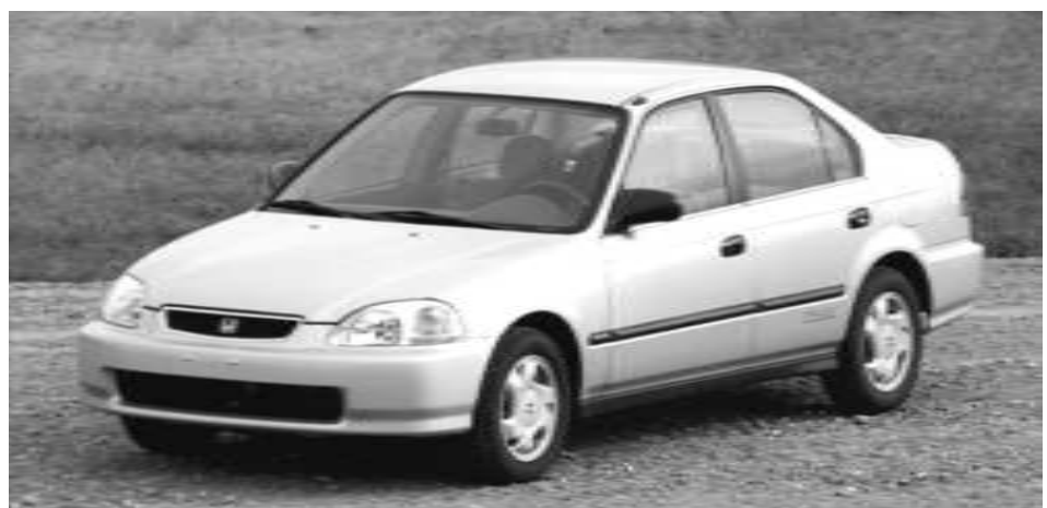
The 1998 Honda Civic GX, a dedicated CNG vehicle, is one of several types tested at the DOE National Renewable Energy Laboratory.
