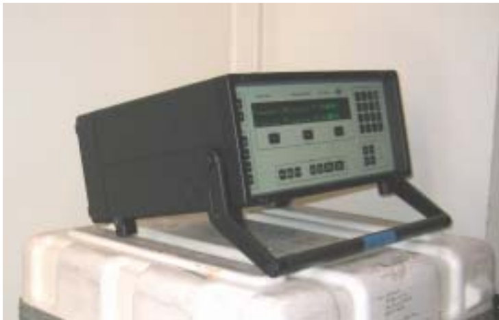
Figure 5-3. The NREL Bruel kjaer photo-acoustic spectrometer is used to measure the SF 6 concentration
