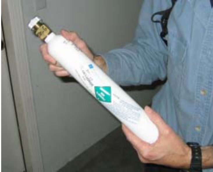
Figure 5-2. The SF 6 tracer gas is released into the garage to provide a starting concentration of 5 to 10 ppm
