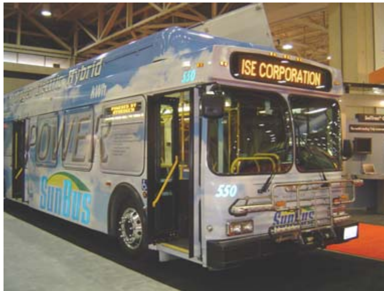
Figure 12. Hydrogen hybrid internal combustion engine bus
