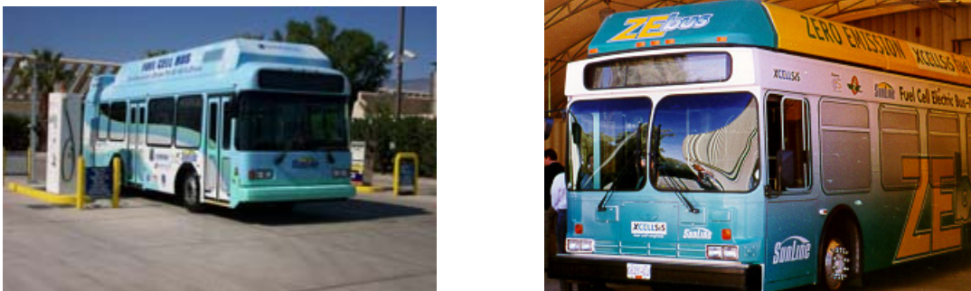
Figure 11. Fuel cell buses tested in operation at SunLine (left – ThunderPower bus with a UTC fuel cell power plant; right – P4 Ballard fuel cell-powered bus)
