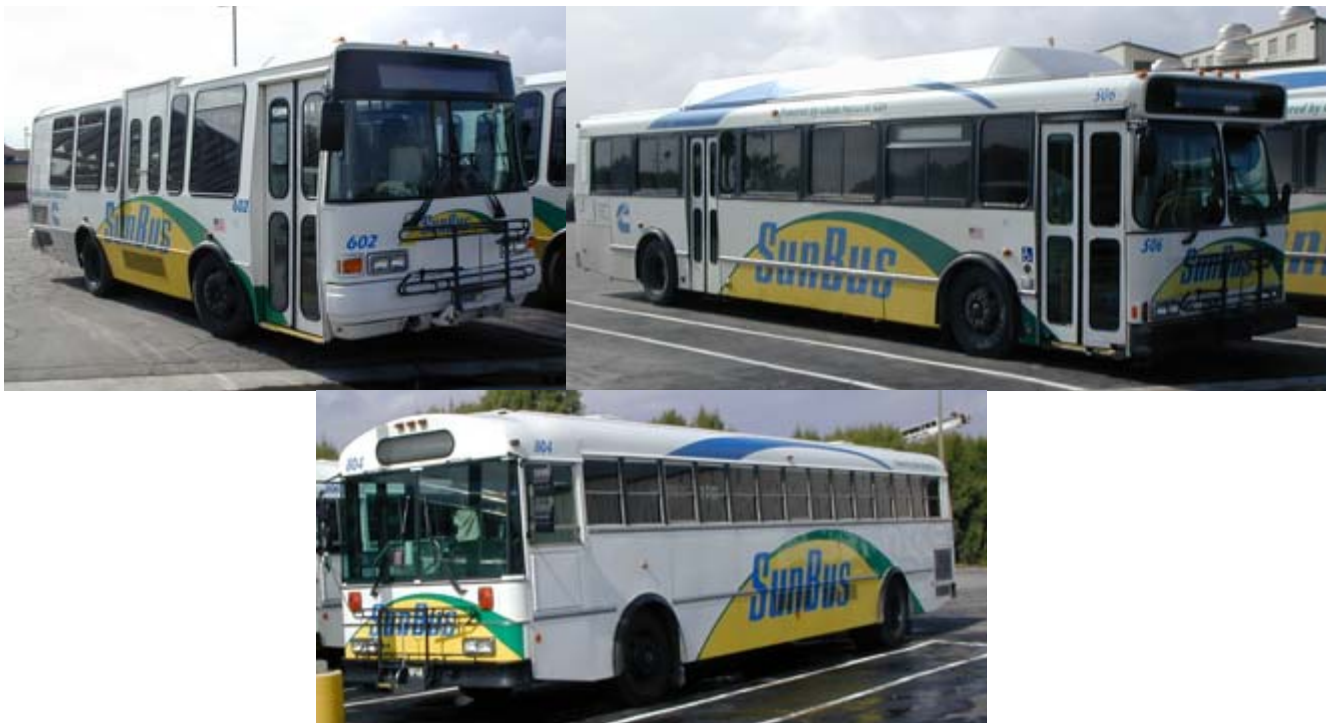
Figure 3. SunLine CNG buses (top left – El Dorado; top right – Orion; bottom – Thomas)
