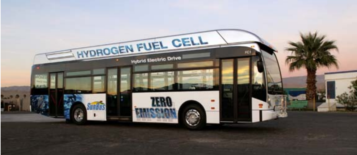
Figure 13. SunLine ISE/Van Hool/UTC fuel cell bus
