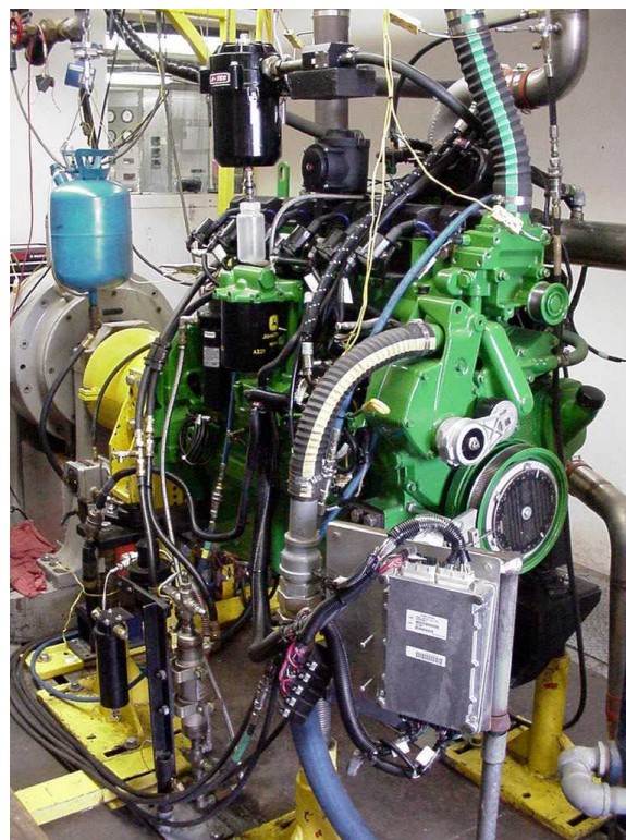
Photo 3-1 and 3-2: John Deere 8.1L deterioration factor engine installed in laboratory dynamometer at SwRI
