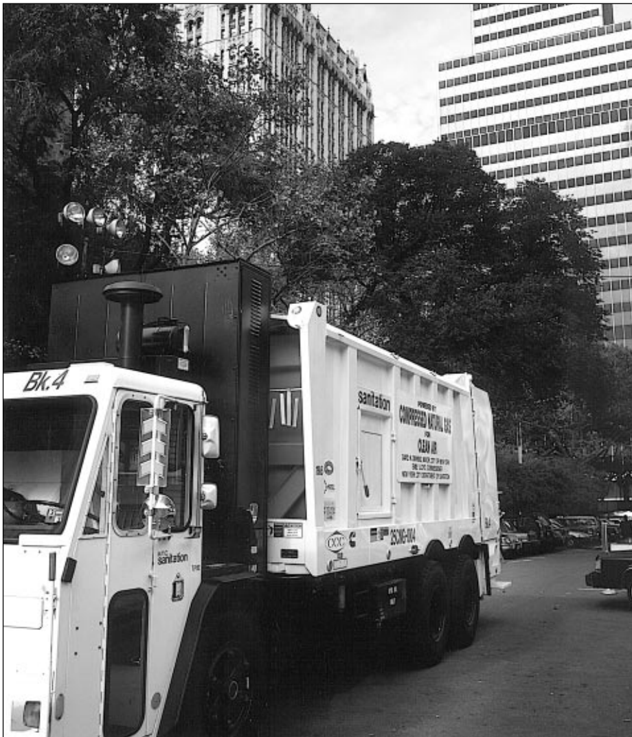
Compressed natural gas refuse hauler on the road in New York City
