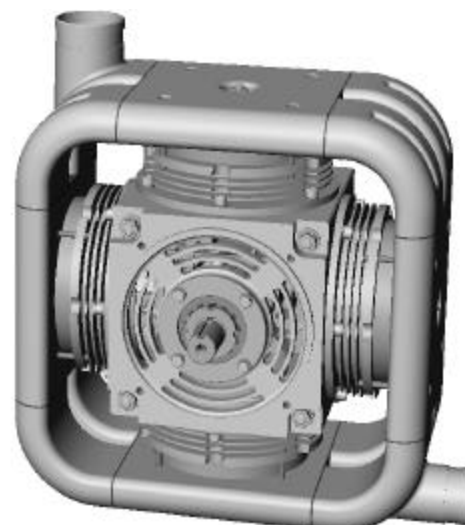
Figure 7. Compressor with manifolds.
