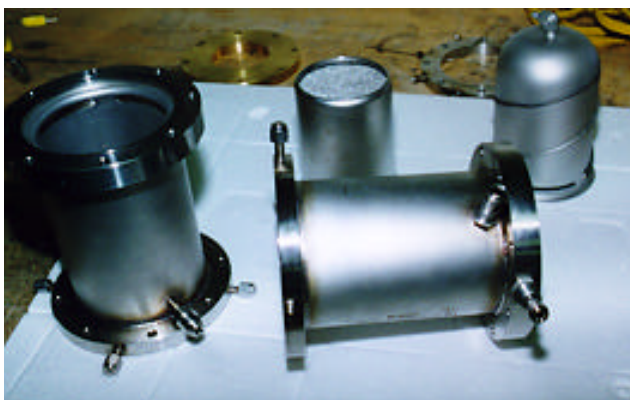
Figure 1. PROX stage components. Outer shell is shown by the two stages in the foreground. A catalyst cartridge is shown in the center background, with a HEX insert in the right background.
