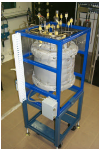
Figure 1. The Fuel-Flexible Fuel Processor (from Hydrogen Burner Technology) at Los Alamos.
