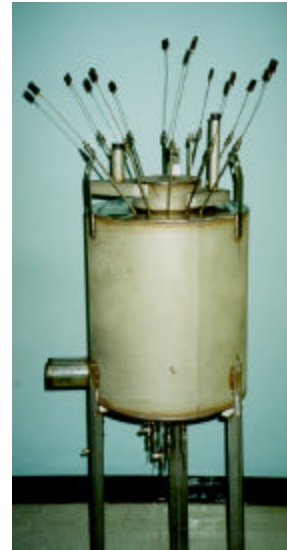
Figure 1. Integrated autothermal reformer test article.
