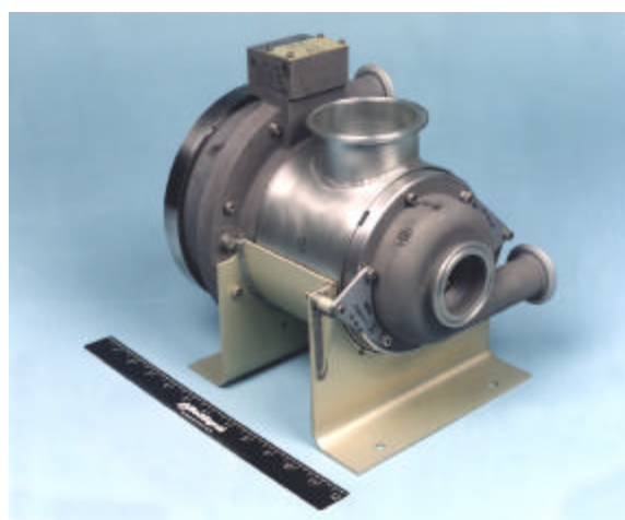
Figure 1. Photograph of turbocompressor.
