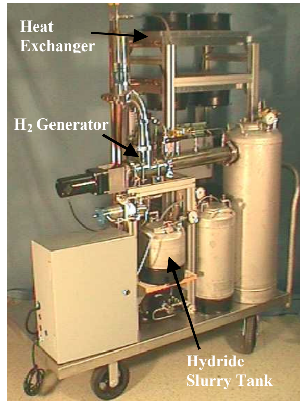
Figure 2. 50-kWe hydrogen generation system.
