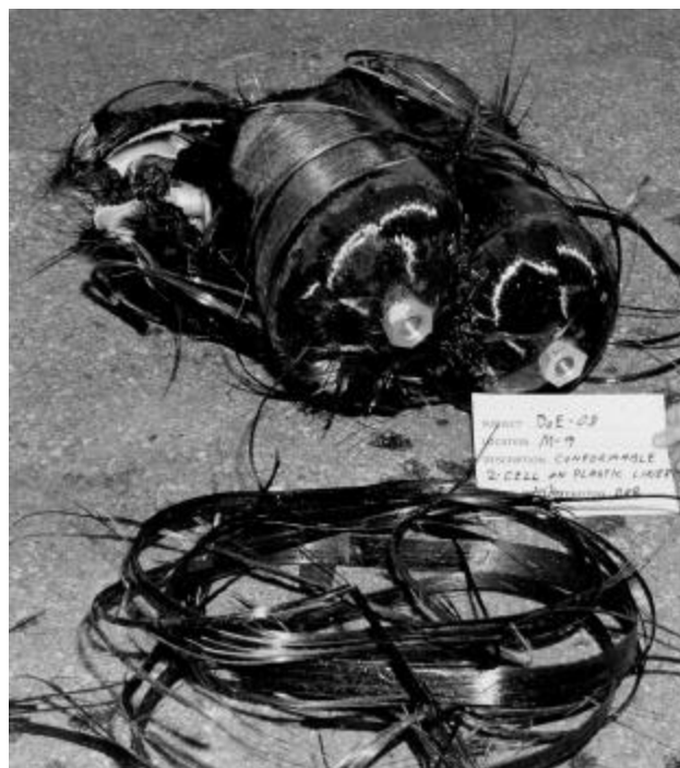
Figure 4. Full-scale conformable tank following hydroburst test.
