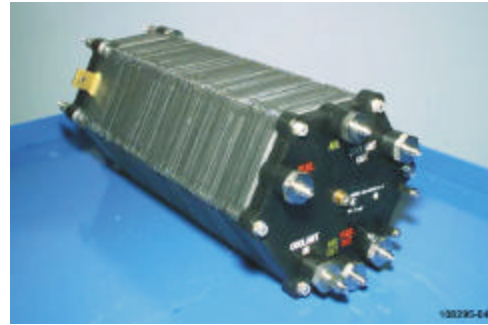
Figure 5. First 10-kW-class stack.
