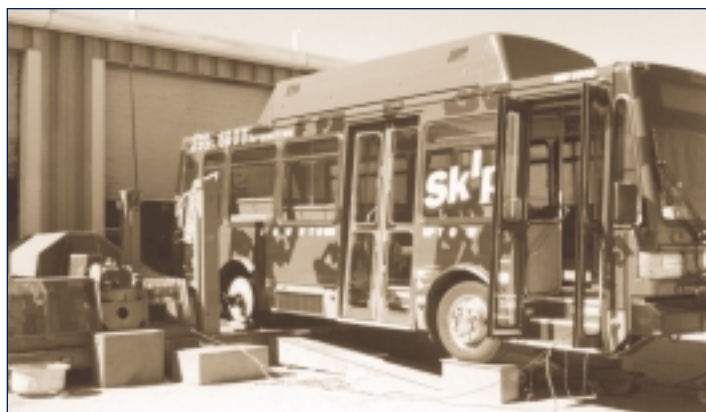
Commercial bus in Boulder, Colorado, being tested on West Virginia University's portable chassis dynamometer
