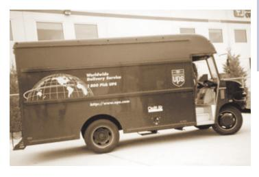
The UPS project, funded by DOE through NREL and managed by TRI, was designed to test the feasibility of using CNG in a "medium-duty" pick-up and delivery fleet. NREL's AFDC has logged data on the fuel use and maintenance requirements of the CNG trucks along with those of similar gasoline-powered trucks.
