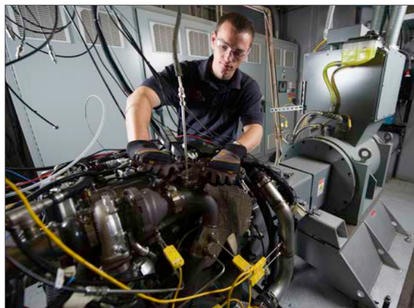
Engine on a dynamometer at the National Renewable Energy Laboratory’s ReFUEL facility. Photo by Dennis Schroeder, NREL 22781
