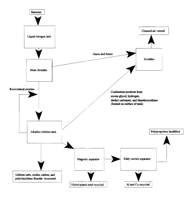
Figure 1. Potential lithium ion battery recycling process
