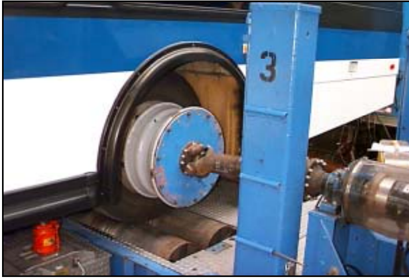
Figure A2: Hub Adapter Connection to the Drive Axle
