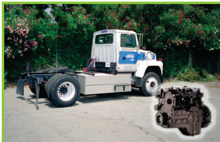
Figure 1. One of two Viking Freight tractor-trailers powered by a C-Gas Plus natural gas engine for the NREL-funded on-road prototype development project. Inset: C-Gas Plus engine.
