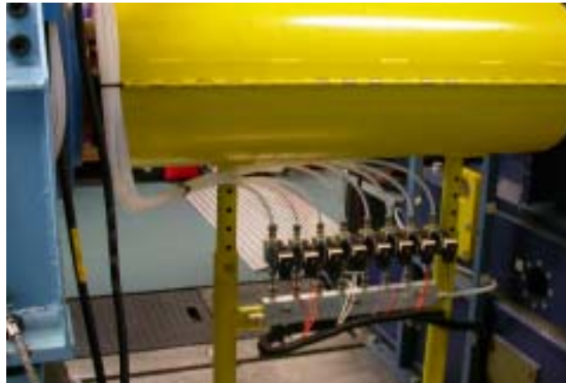
Figure 54: EGR Sample Switching Manifold
