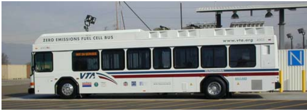
Figure 1. Fuel Cell Transit Bus at VTA
