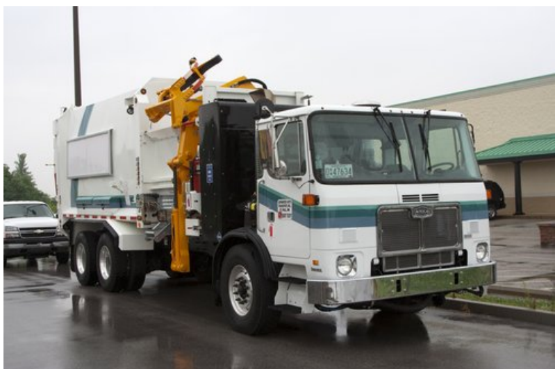
A CNG-powered refuse truck in Indiana. Slow-fill or time-fill CNG fueling systems are appropriate for vehicles that park overnight in a central location.
