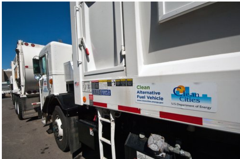
A refuse hauler fueled with B20—20% biodiesel, 80% petroleum diesel. Biodiesel is a renewable fuel and produces lower levels of greenhouse gas emissions than regular diesel. Photo by Pat Corkery, NREL/PIX 18124
