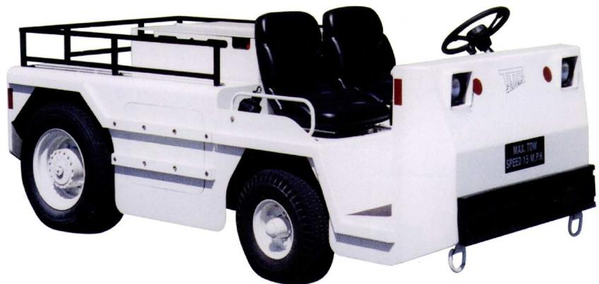
*An electric tow tractor like this one pulls a wagon used for maintenance work in the Redwood National & State Parks. The quiet operation ensures the wildlife will not be disturbed.*
