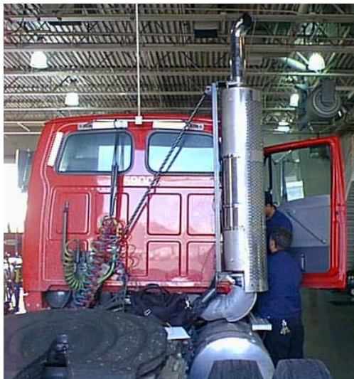
Figure 4. Ralphs Grocery Truck with DPF Installed (Left) and Johnson Matthey CRT (Right)
