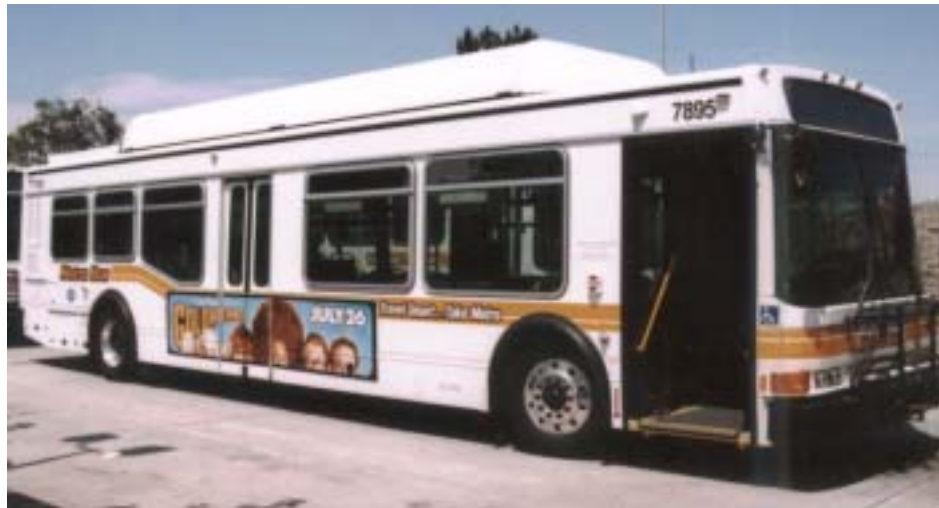
2002 NABI 40 ft low floor CNG transit bus used by Los Angeles County MTA
