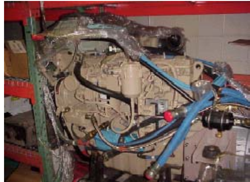
Cummins-Westport C Gas Plus Heavy-Duty Natural Gas Engine (photo from Pierce Transit)
