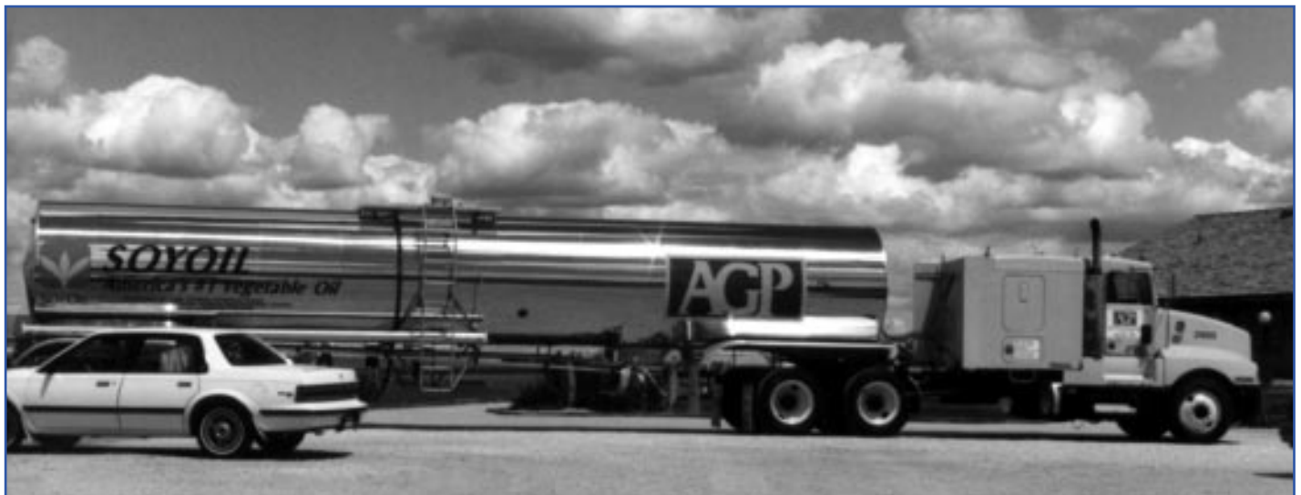
This tractor in AGP's fleet runs on a blend of 65% petroleum diesel and 35% soybean methyl esters (biodiesel).
