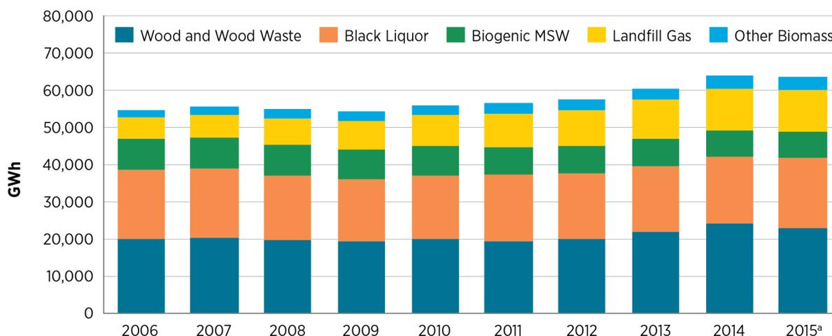
**Figure 33. U.S. biopower generation sources**
