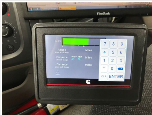
FIGURE 4 Human-Machine-Interface for driver to enter the mission distance
