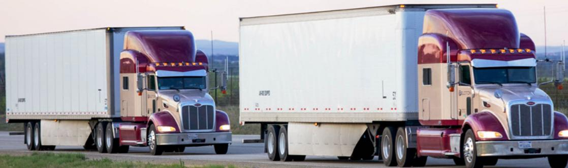
NREL researchers are evaluating truck platooning, a strategy to reduce aerodynamic drag by grouping tractor trailers closely together on the highway. *Photo from Peloton, NREL 31237*
