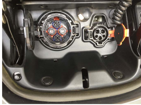
Figure 10. Under the plug cover of a Nissan LEAF, showing a J1772 charging plug for AC Level 1 and Level 2 charging (right) and a CHAdeMO charging plug for DCFC (left).
