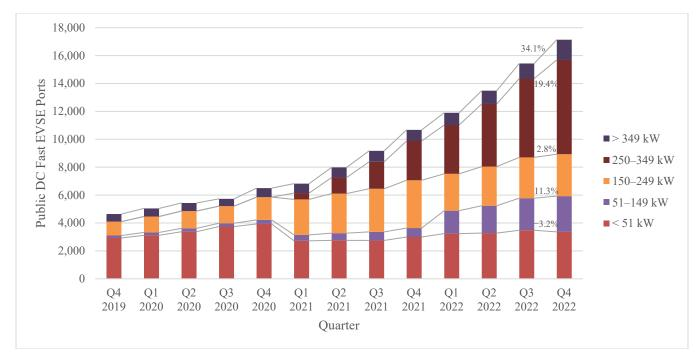
Figure 6. Quarterly growth of public DC fast EVSE ports by power output.
