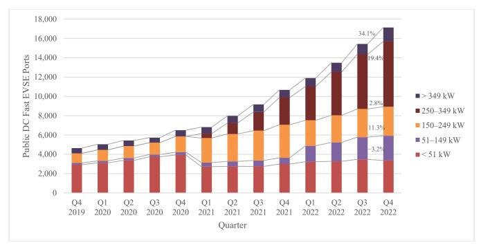
Figure ES-3. Quarterly growth of public DC fast EVSE ports by power output.
