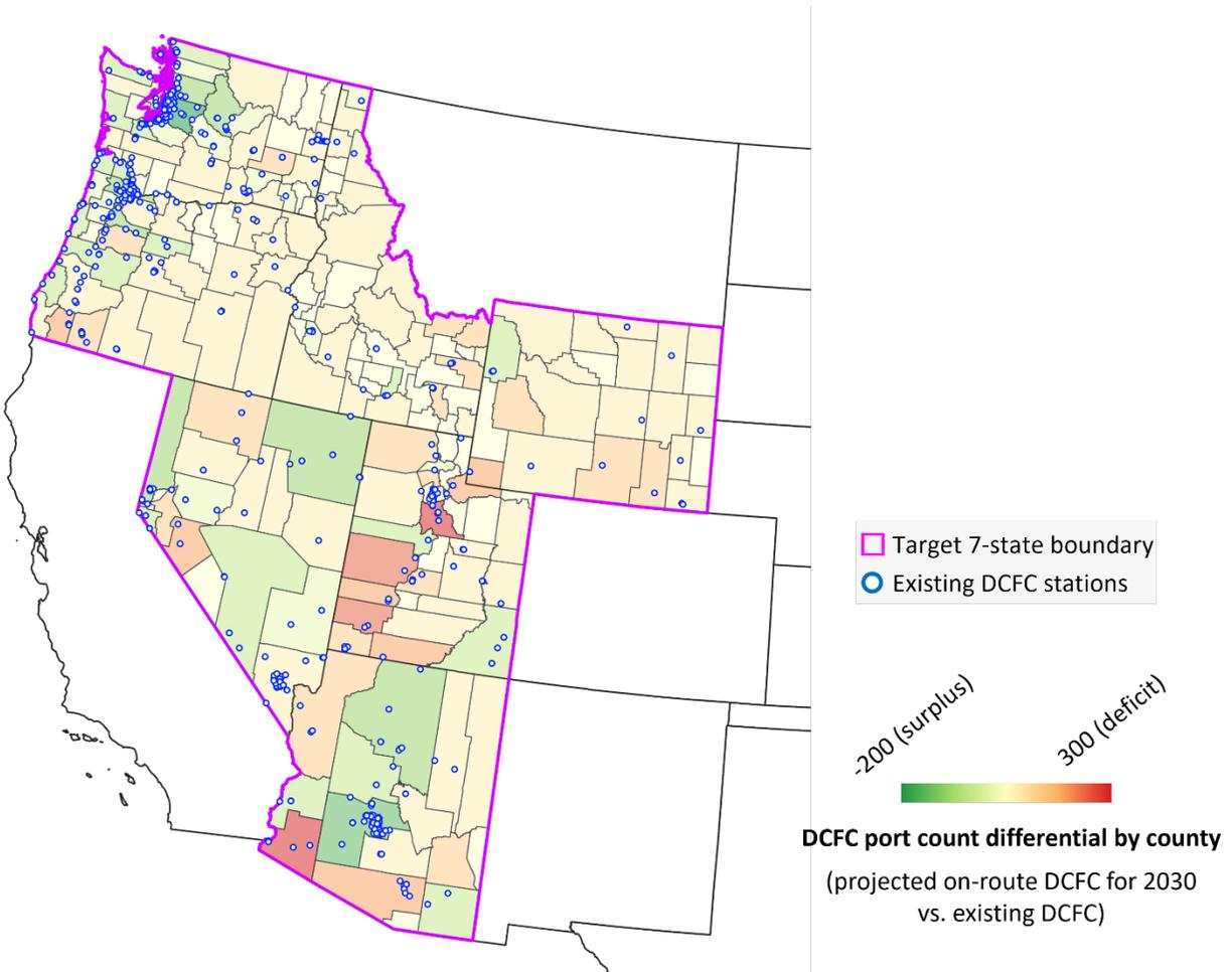
**Figure 11. County-by-county DCFC port count differential (negative: surplus; positive: deficit) between projected on-route DCFC for 2030 vs. existing DCFC**
