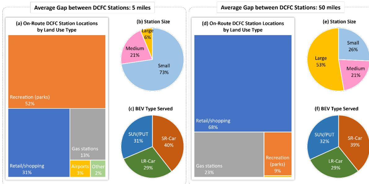
**Figure 15. Land use type, station size, and BEV type served for two different settings for the average gap between stations—5 miles (left: a, b, and c) vs. 50 miles (right: d, e, and f)—for the simulated network of on-route DCFC stations in the seven states in 2030 (Figure 10)**
