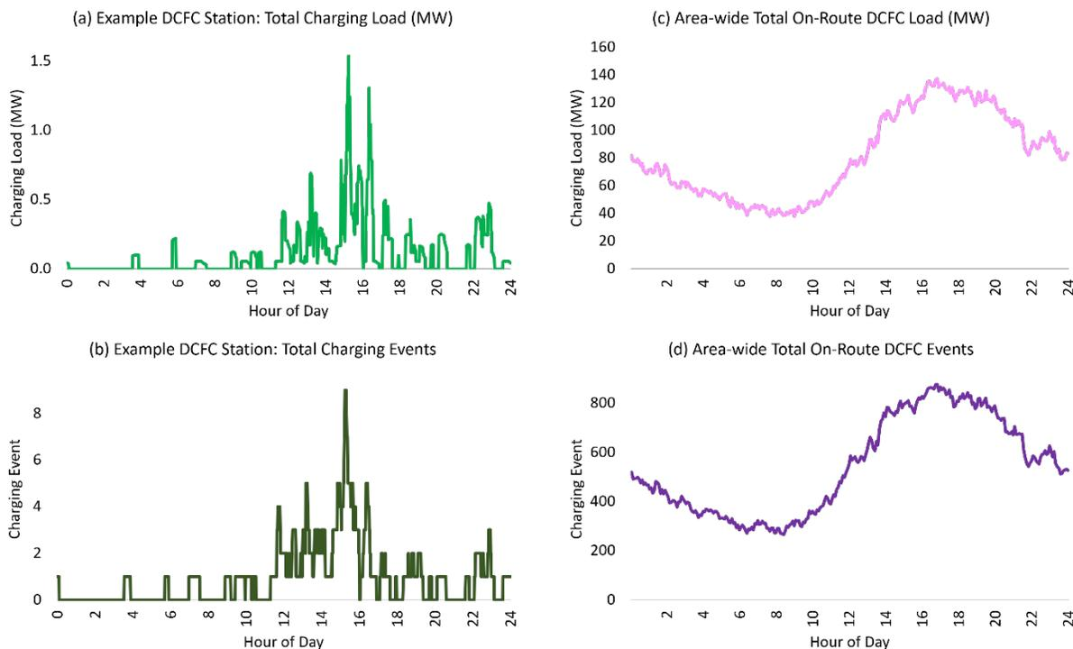
**Figure 16. (a) Site-level on-route DCFC load profiles and (b) total charging events; (c) and area-wide charging load profiles and (d) total charging events for the scenario of high BEV penetration, TPM charging behavior, and 50-mile gaps between stations in 2030**
