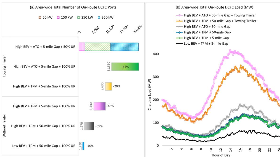
**Figure 17. (a) The numbers of required on-route DCFC ports in 2030 and their variations according to different scenarios/assumptions. (b) Total on-route charging load profiles in the study area in 2030, depending on various scenarios/assumptions**
