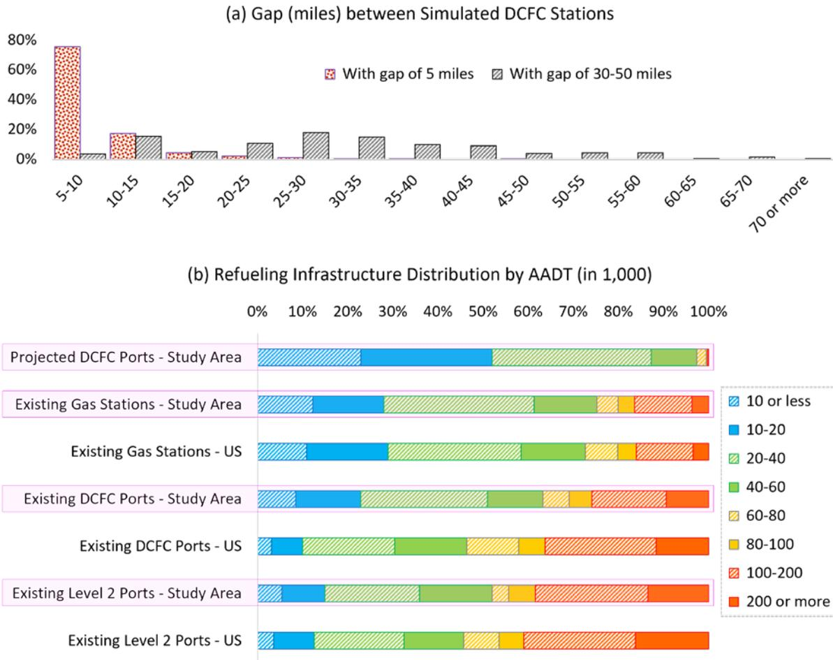
**Figure 12. (a) Distribution of the gaps (miles) between DCFC stations for two different scenarios: 5 miles vs. 50 miles. (b) Relationship between the concentration of the refueling infrastructure (in the study area vs. the United States) and the AADT as a proxy of the level of vehicle activity**
