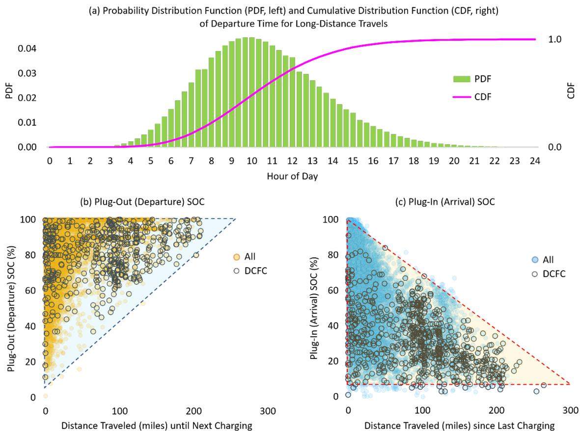
**Figure 4. (Top) Probability distribution function (PDF) and cumulative distribution function (CDF) for departure time for road trips based on travel surveys on long-distance travelers. (Bottom) Empirical relationship between plug-in and plug-out SOC as a function of pre-/post-charging distance traveled/driven**
