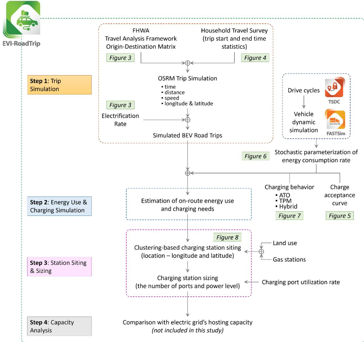
**Figure 2. Schematic diagram of EVI-RoadTrip**
