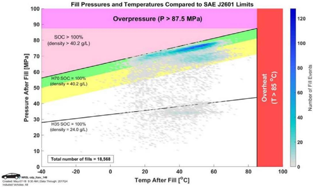
Figure 11. Fill pressures and temperatures compared to SAEJ2601 (CDP-FCEV 149)
