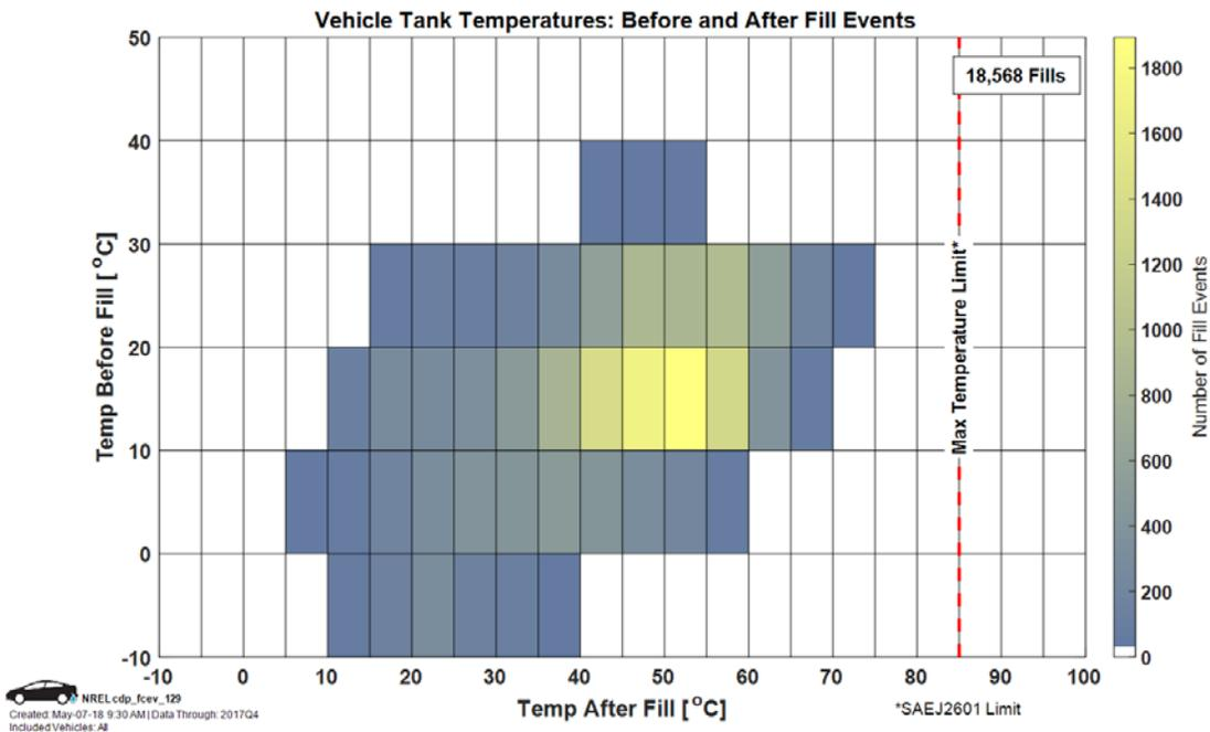
Figure 12. Vehicle tank temperature: before and after fill events (CDP-FCEV 129)
