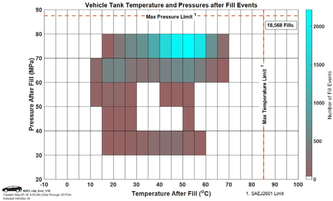
**Figure 13. Vehicle tank temperature and pressure after fill events (CDP-FCEV 130)**
