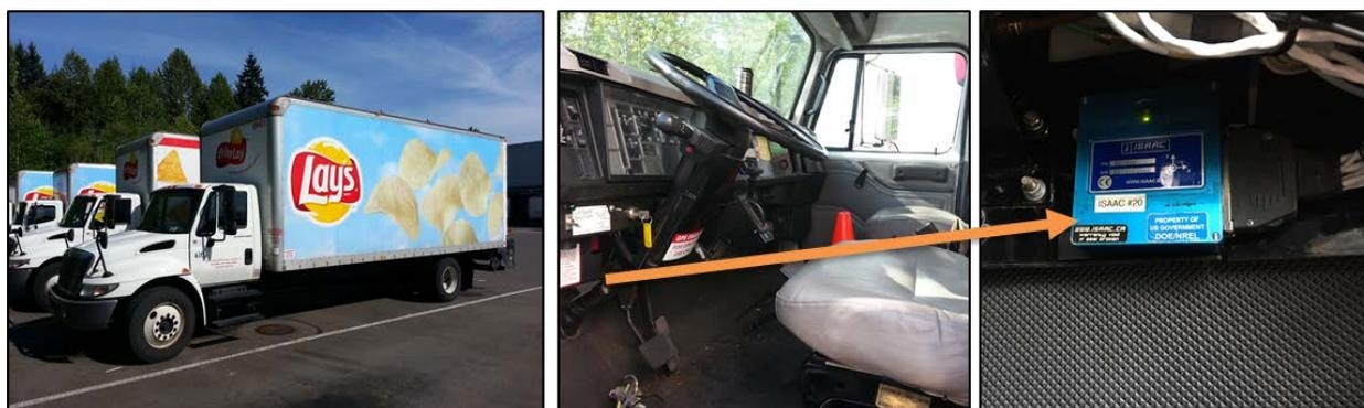
Figure 6. Diesel vehicle data logger installation (Photos by Adam Ragatz, NREL)
