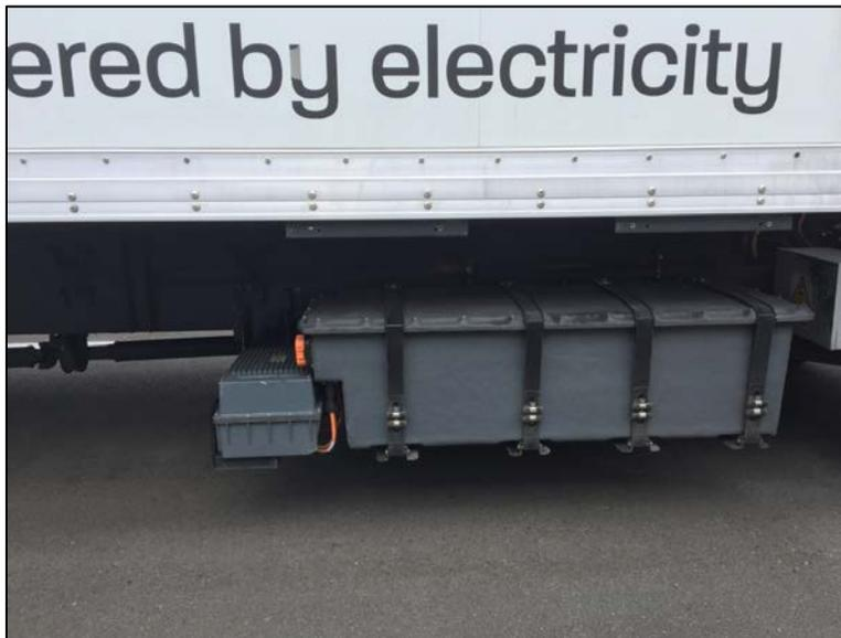
**Figure 4. Smith Newton with passenger-side aerodynamic skirting removed showing 80-kWh LiFePO<sub>4</sub> battery pack (Photo: Robert Prohaska / NREL)**
