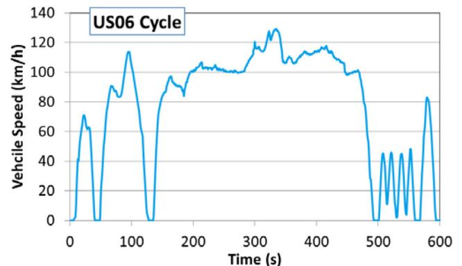
Figure 8. The US06 drive cycle represents relatively aggressive, but realistic, driving.
