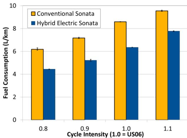
Figure 18. Experimental FC results for the conventional and hybrid Hyundai Sonatas as a function of US06-based cycles with altered intensity levels.
