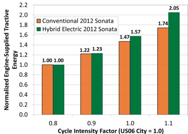
Figure 15. Normalized engine-supplied tractive energy as a function of US06 City-based drive cycle.
