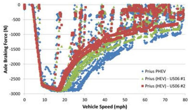
Figure B1. RB force over two consecutive US06 cycles (green and red points) for a 2010 Toyota Prius. Data are also shown for a 2012 Prius PHEV. Figure is courtesy of Argonne [22, 24].
