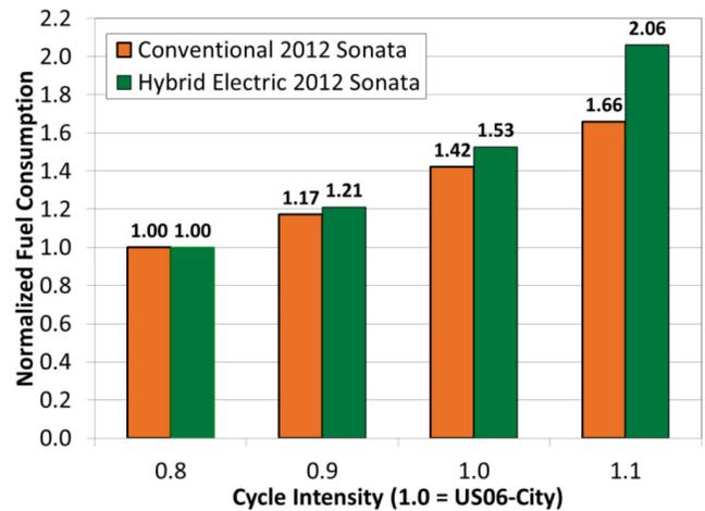
Figure 21. Normalized FC results for the conventional and hybrid Hyundai Sonatas as a function of US06 City-based cycles with altered intensity levels.
