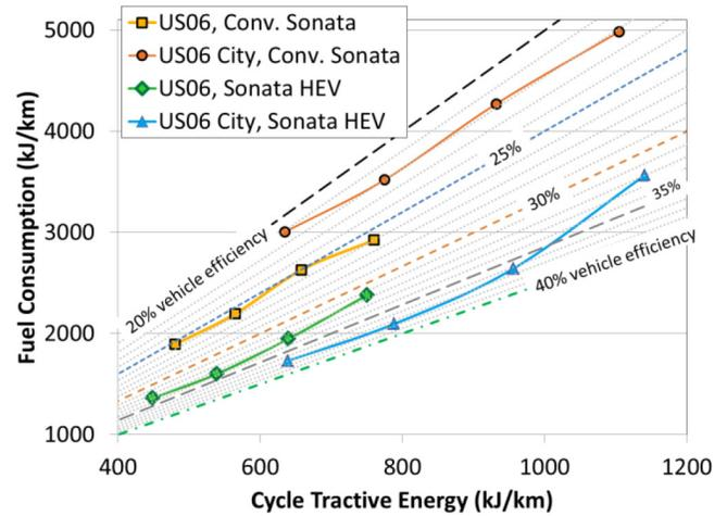
Figure 24. Fuel energy as a function of tractive energy for the conventional and hybrid Hyundai Sonatas over intensity modified US06 and US06 City cycles.
