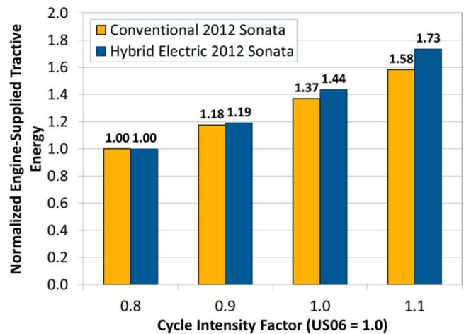
Figure 14. Normalized engine-supplied tractive energy as a function of US06-based drive cycles.
