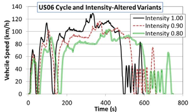
Figure 11. The US06 cycle can be modified in intensity to form variants with lower or higher speeds and rates of accelerations and decelerations.
