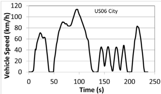
Figure 13. The US06 City cycle is shown here as one continuous cycle.
