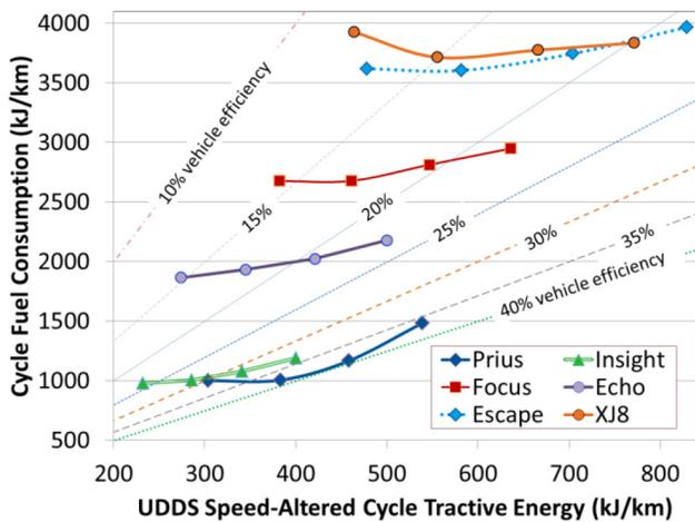
Figure 25. Fuel energy as a function of tractive energy for six vehicles for speed multiplied UDDS cycles in [10] (speed multipliers are 0.8, 1.0, 1.2, and 1.4).
