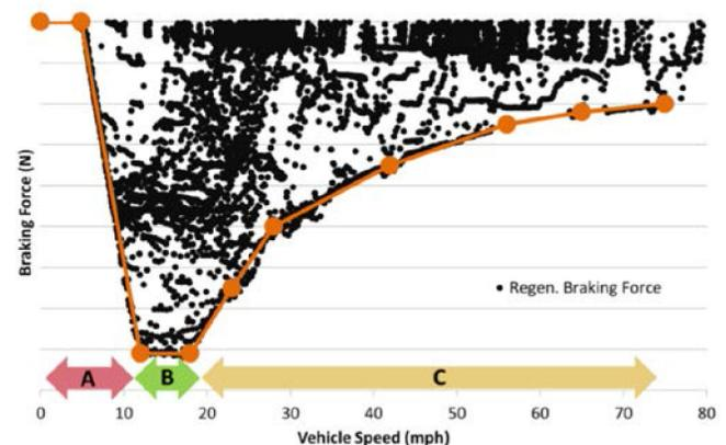
Figure 7. RB limitations (used by permission, Rask et al. [16]).
