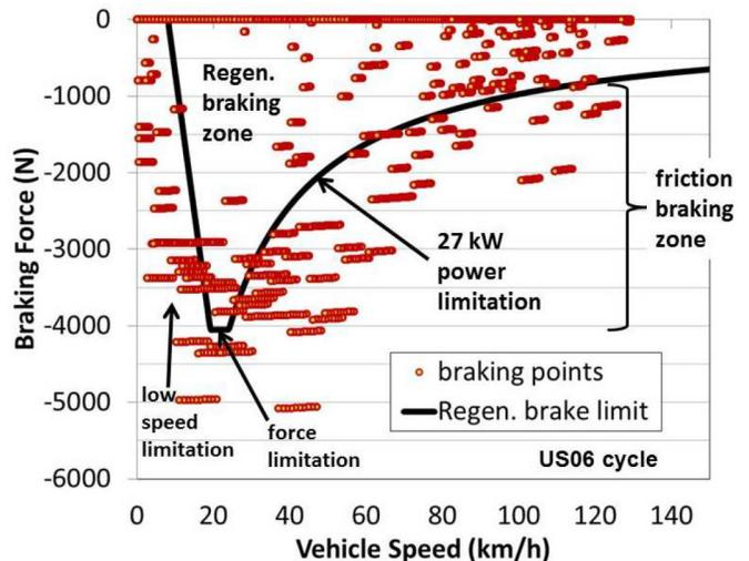
Figure 9. RB limits for a 2011 Sonata HEV and calculated brake force needed over the US06 cycle.
