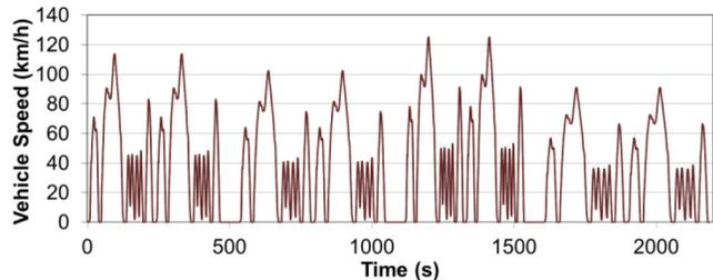
Figure 17. US06 City-based cycles are shown in the experimental sequence used for the conventional vehicle with intensity scaling factors of 1.0, 0.9, 1.1, and 0.8, respectively. The sequence features pairs of identical cycles to create a longer drive length for each condition.
