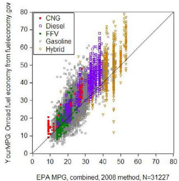
Figure 1. Self-reported miles per gallon (mpg) values from [www.fueleconomy.gov](http://www.fueleconomy.gov) plotted against the EPA label values. CNG = compressed natural gas; FFV = Flexible Fuel Vehicle
