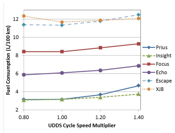
Figure 4. Results for FC for six vehicles tested over the UDDS cycle and intensity variant cycles altered by speed multipliers [10].
