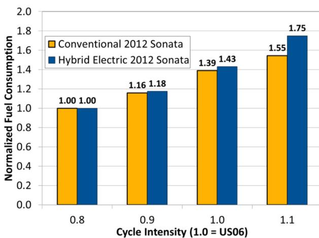
Figure 20. Normalized FC results for the conventional and hybrid Hyundai Sonatas as a function of US06-based cycles with altered intensity levels.
