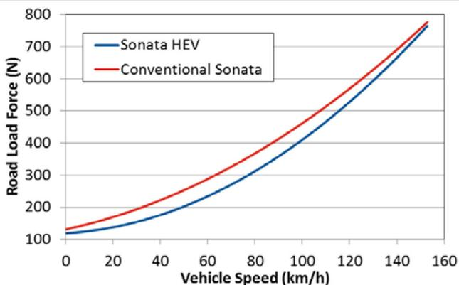
Figure 10. Road-load force curves for the 2011 Hyundai Sonata hybrid and conventional vehicles.
