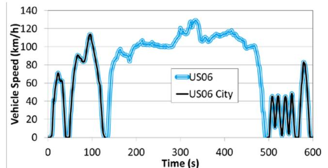
Figure 12. The US06 City cycle is represented by the two portions of the US06 trace shown in black. The US06 City cycle retains much of the hard accelerations and decelerations of the US06.
