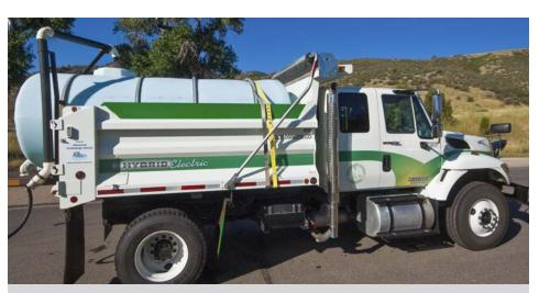
HEVs work well for both light-duty and heavy-duty applications, particularly those that require frequent stops and starts. *Photo by Pat Corkery, NREL 18142*
