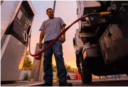
CNG vehicles are fueled with easy-to-use, pressure-sealed fueling dispensers. Photo by Dennis Schroeder, NREL 48723
