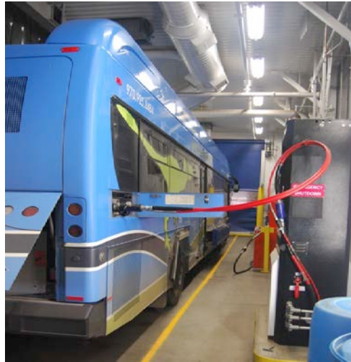
Figure 4. VelociRFTA bus at indoor CNG fueling facility. Photo by George Mitchell, NREL 34949
