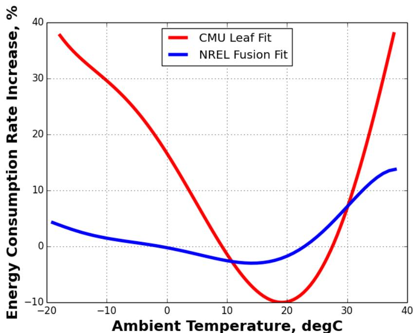
Figure 15. Relative energy consumption rate increase as a function of ambient temperature. Carnegie Mellon University fit to battery electric Nissan Leaf data (red) and NREL fit to conventional spark-ignited gasoline Ford Fusion simulations (blue).
