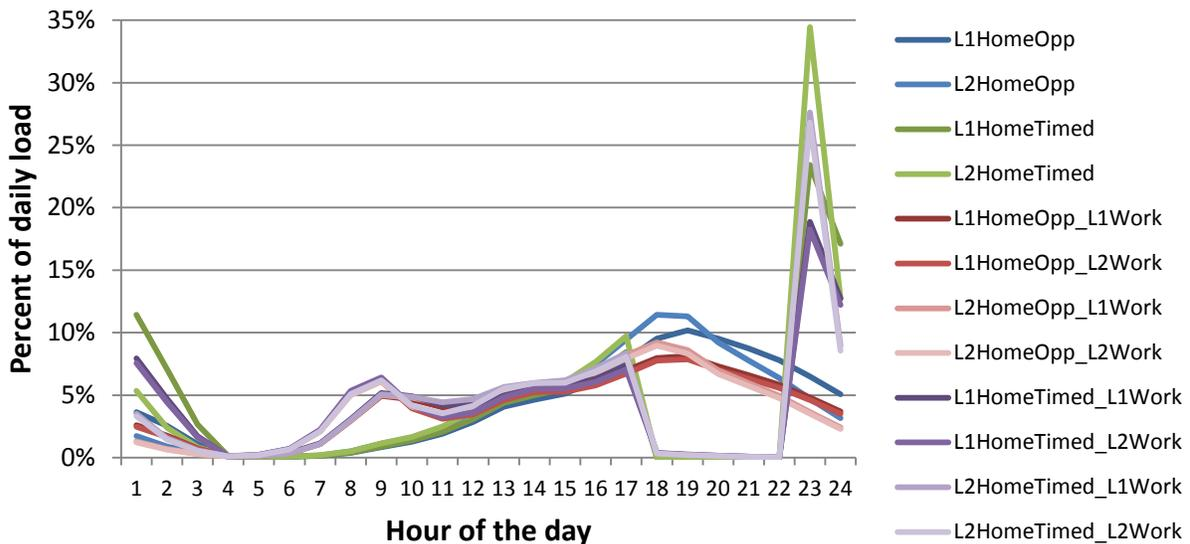
**Figure 29. Charging profiles for various charger sizes and configurations**
