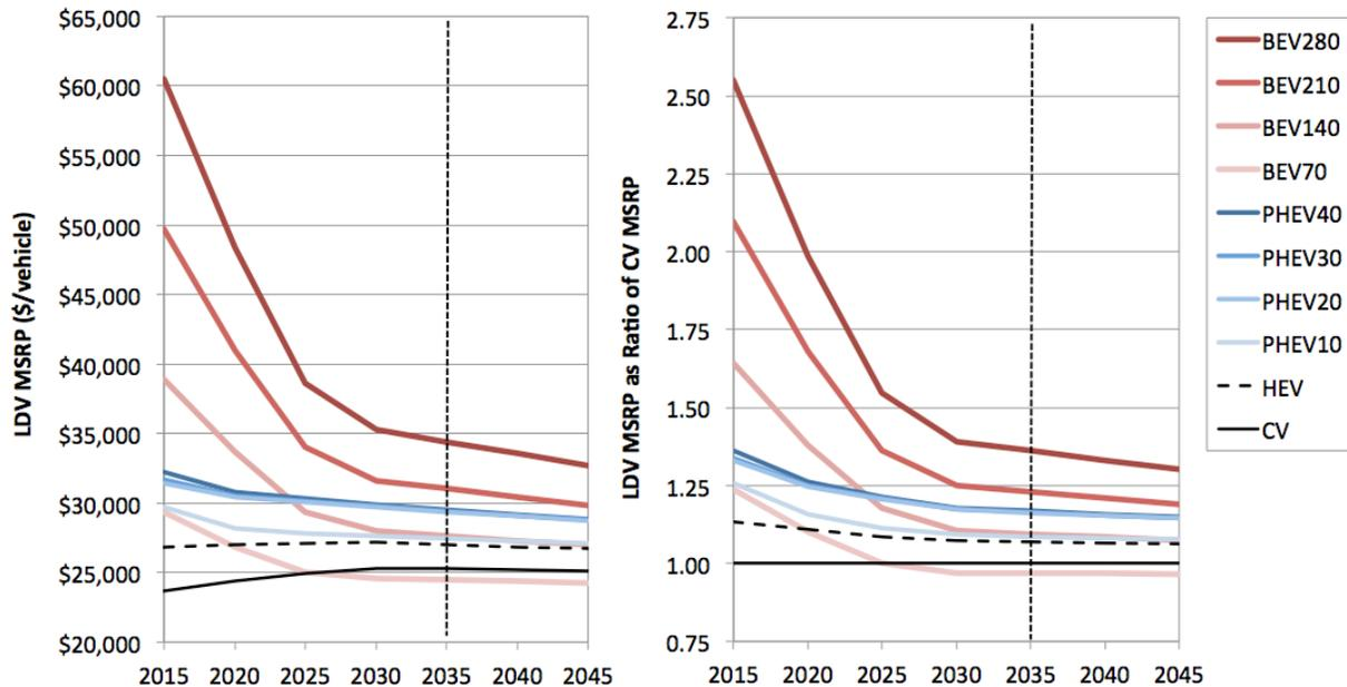
**Figure ES-2. Time series representation of the high-med light-duty vehicle BaSce cost trend results from Moawad et al. (2016), after applying a 1.5 retail markup factor to estimate the manufacturer’s suggested retail price (MSRP), shown in units of dollars per vehicle (left) and as a ratio of CV retail prices (right)**
