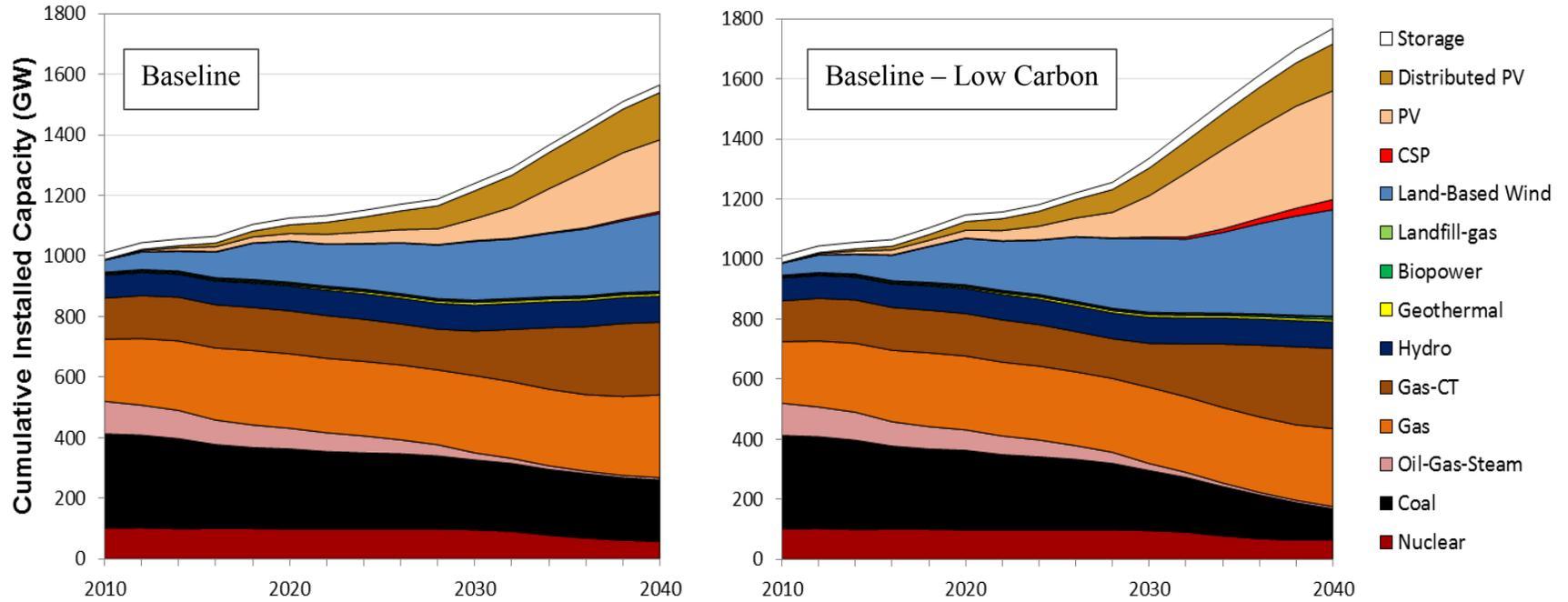
Figure 41. Cumulative capacity by generation technologies: Baseline and Baseline-Low Carbon
