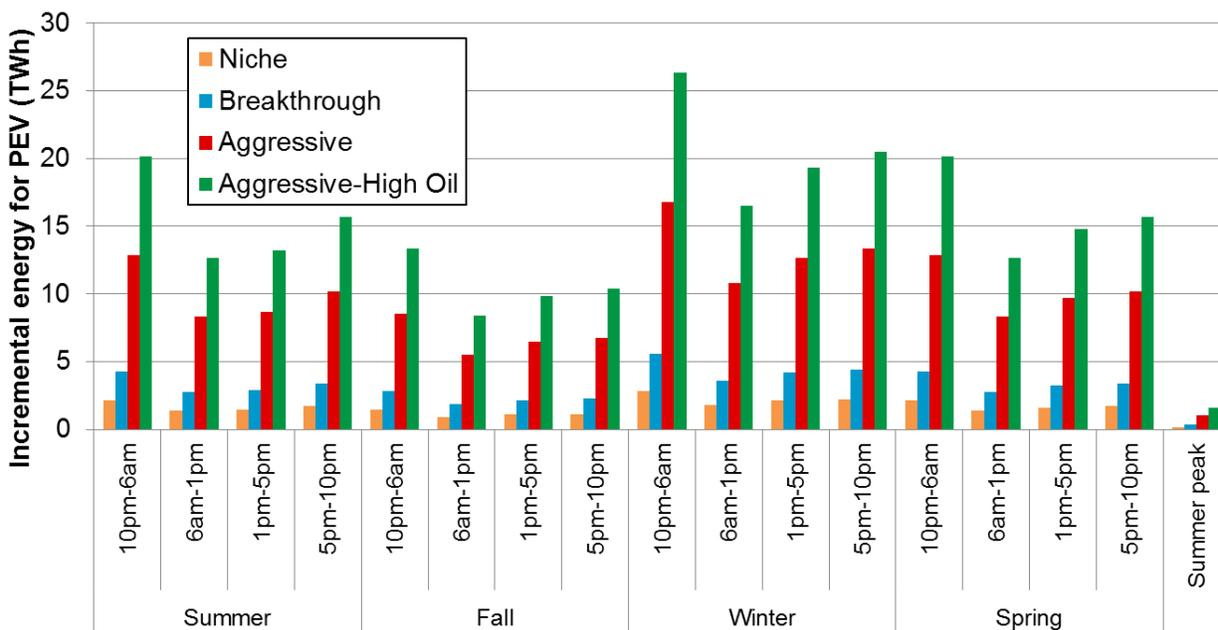
Figure 38. Additional energy demand imposed by PEVs in 2035 by ReEDS time slices
