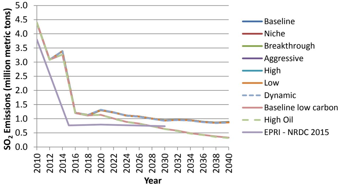
Figure 49. SO<sub>2</sub> emissions for the U.S. electric sector for each scenario of vehicle electrification
