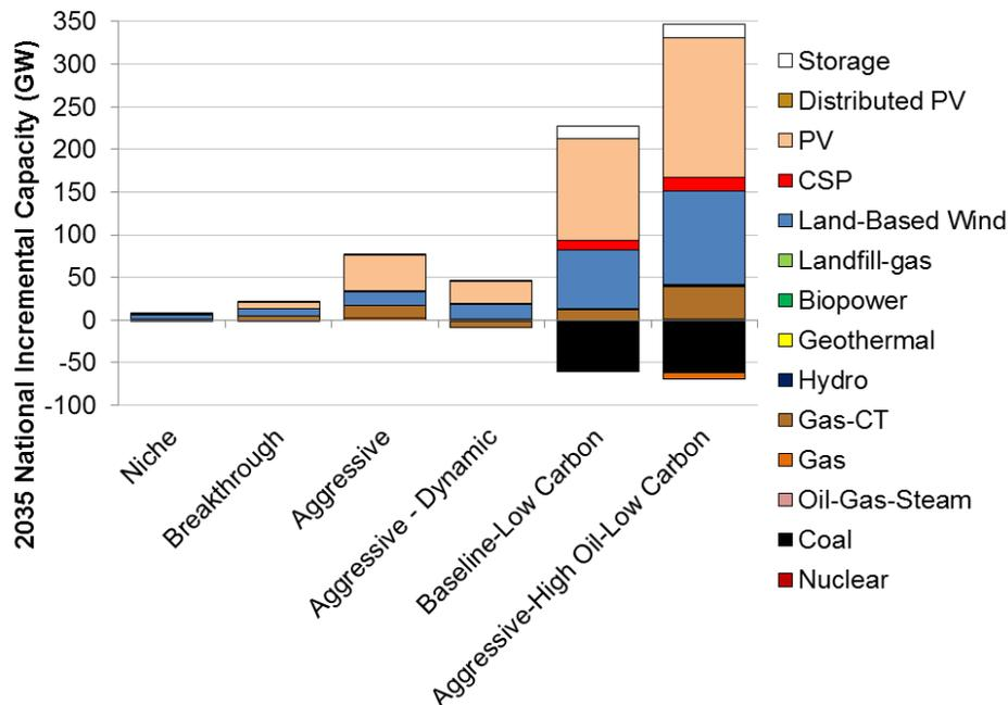
**Figure ES-5. Year 2035: Incremental installed electricity generation capacity compared to the Baseline scenario**
