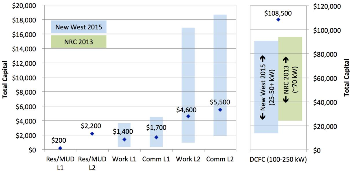
**Figure 17. Total equipment and installation capital costs for EVSE by type and location**
