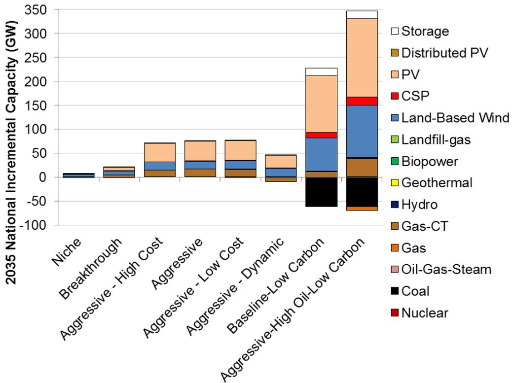
Figure 43. Year 2035: Incremental installed capacity compared to the Baseline scenario
