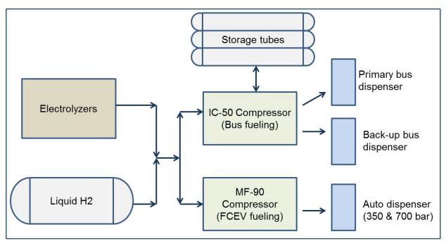
Figure 7. Block diagram of the Emeryville station
