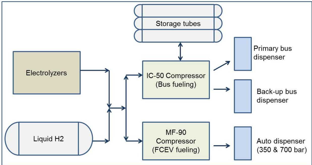
**Figure 7. Block diagram of the Emeryville station**
