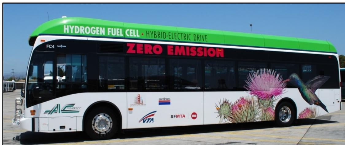
**Figure 3. AC Transit fuel cell bus**
