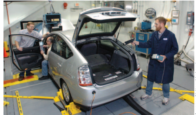
PHEV chassis dynamometer testing at Argonne National Laboratory’s Advanced Powertrain Research Facility.
