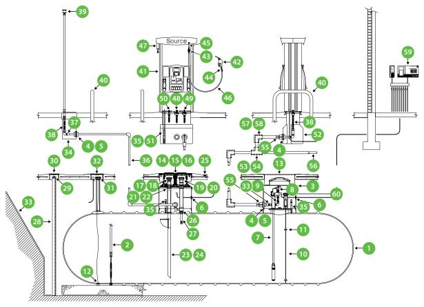
Figure 2. Typical Fuel Dispenser and Underground Storage Piping. Illustration by Source North America
