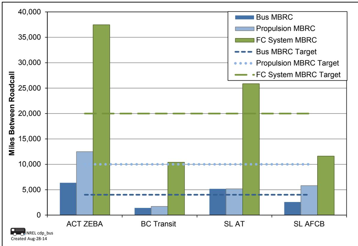
**Figure 8. MBRC rates for FCEBs compared to the targets**
