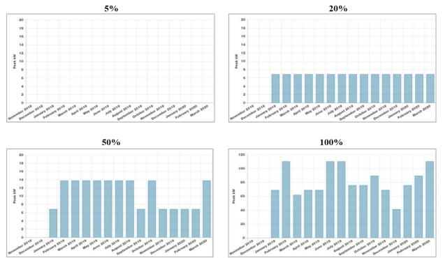
Figure E-1. Projected monthly peak charging demand at increasing levels of fleet electrification for a single parking facility: UT Knoxville
