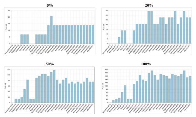
Figure F-1. Projected monthly peak charging demand at increasing levels of fleet electrification for a single parking facility: UVA
