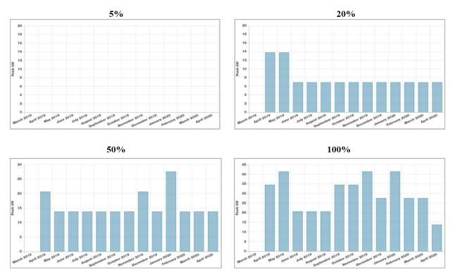
Figure B-1. Projected monthly peak charging demand at increasing levels of fleet electrification for a single parking facility: UCLA
