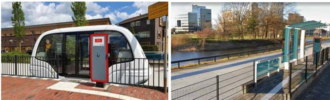
**Figure 3-27. Precision docking allows wheelchair-level platform boarding at station berths.**
