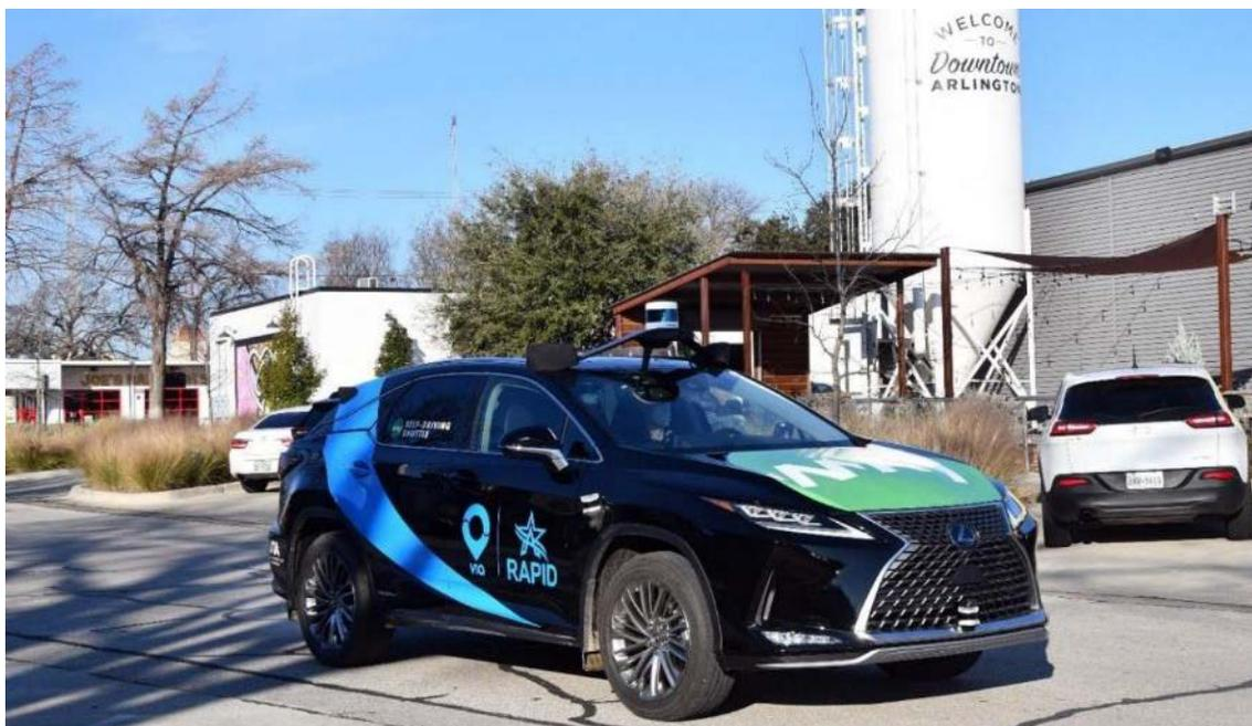
**Figure 3-5. May Mobility deployed Lexus RX450h vehicles augmented by their ADS technology.**
