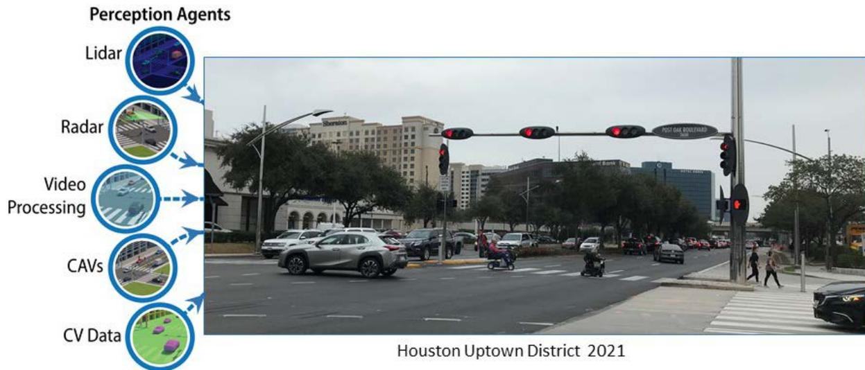
**Figure 5-2. Sensing and perception agents proposed for roadway infrastructure applications**
