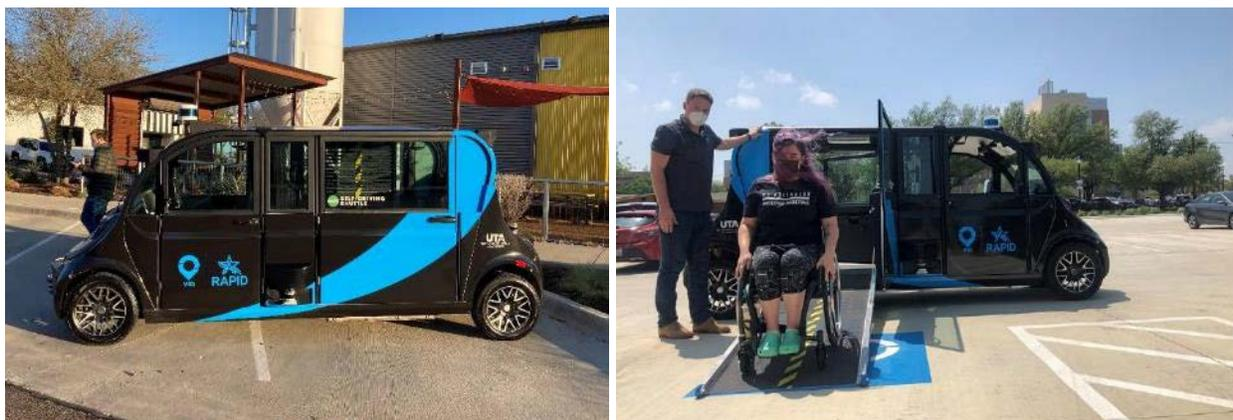
**Figure 3-6. May Mobility's Polaris GEM AV shuttle for wheelchair-accessible service.**
