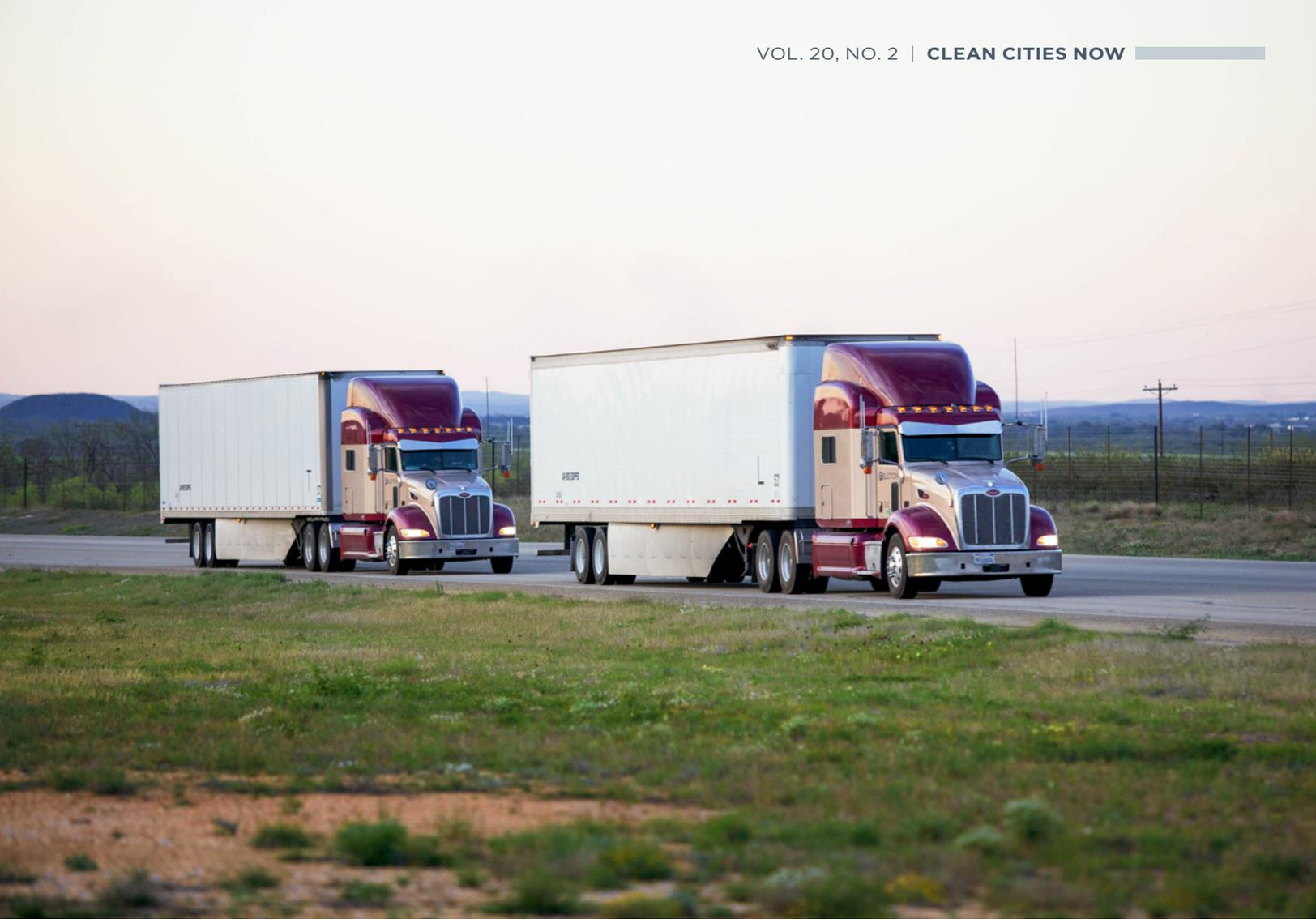
NREL researchers are evaluating truck platooning, a strategy to reduce aerodynamic drag by grouping tractor trailers closely together on the highway. *Photo from Peloton, NREL 31237*
