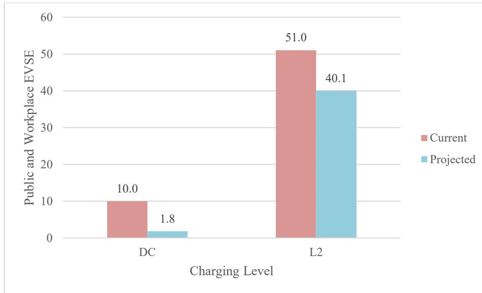
**Figure 16. Current availability and projected 2030 need of public and workplace EVSE per 1,000 EVs in the United States.**
