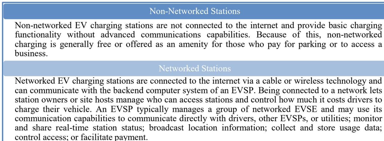
**Figure 1. Non-networked vs. networked EV charging stations.**
